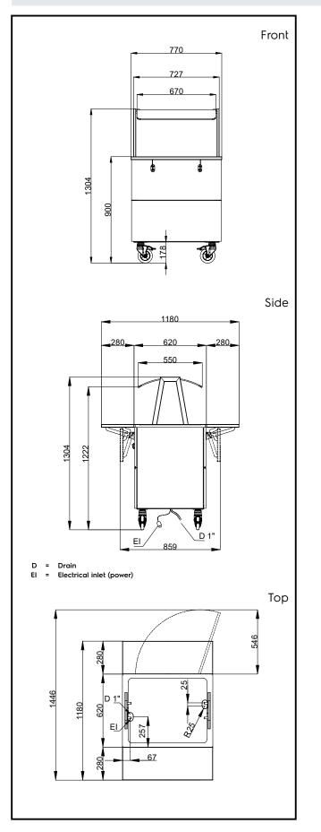
Flexy Compact Refrigerated well on cupboard, static with fan (2GN) with wheels, overshelf with LED lights, H=900mm The company reserves the right to make modifications to the products without prior notice. All information correct at time of printing.
